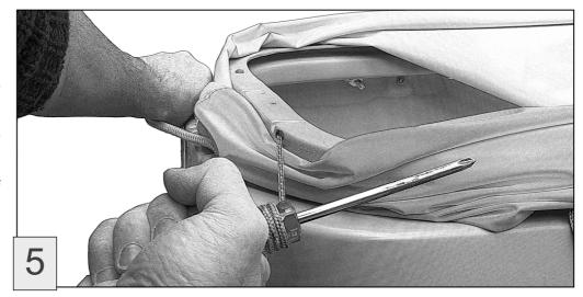
Unzip the cover. Working from inside the sled tie a stopper knot in the cord below the cleat (a). Thread the other end of the cord through the pulley wheel (b). You may need to push the cord thorough with a small screwdriver.
